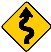
Winding road ahead.
