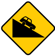
Steep descent (down grade) ahead.
