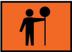
Traffic controller ahead. Be prepared to stop.
