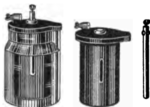
FIG. 222.—The Leclanché cell, "wet" type.
