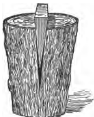
FIG. 102.—One use of the wedge.
