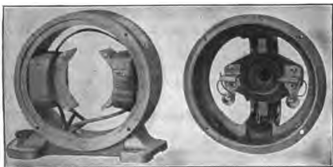
FIG. 300.—The frame and electromagnet (at left), front bracket and brush holder (at right) of the motor shown in Fig. 299.
