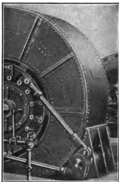
FIG. 116.—The outer case of a turbine showing the mechanism for controlling the gates.
