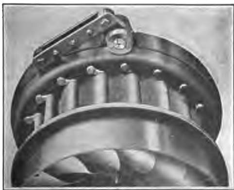
FIG. 117.—Inner case of a turbine showing the gates and the lower end of the runner within.
