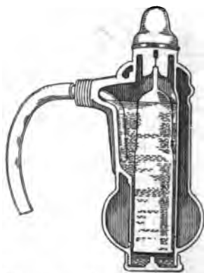
FIG. 145.—An automatic air valve.
