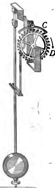
FIG. 82.—Escapement and pendulum of a clock.
