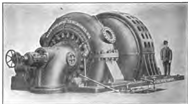
FIG. 119.—Turbine and generator of the Tacoma hydro-electric power plant.
