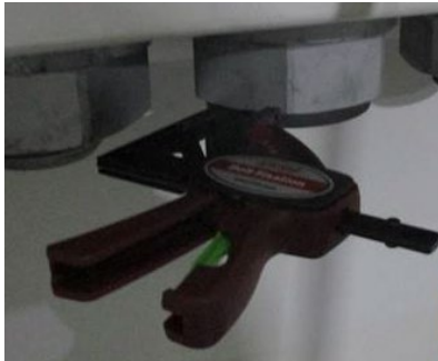
Figure 9.1 – Photographic example of a correctly secured stud thread holder/bolt fixation tool
