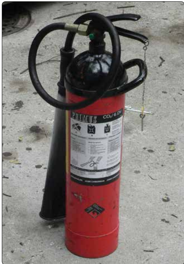
Figure 1-4. Carbon dioxide fire extinguisher.
