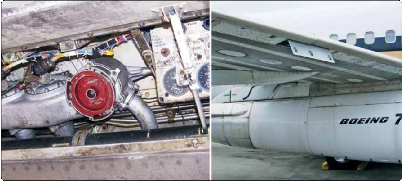
Figure 1-33. Single point refueling station of a large aircraft.
