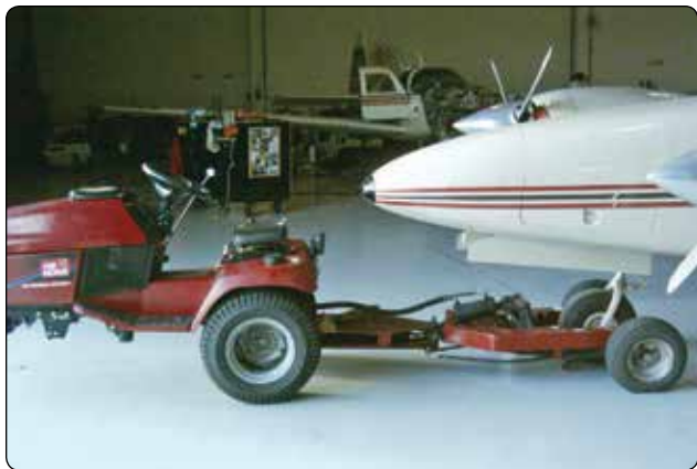
Figure 1-21. Typical smaller aircraft tow tractor.
