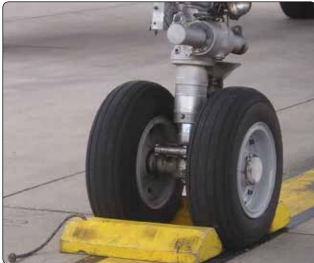
Figure 1-12. Wheels chocked fore and aft.
