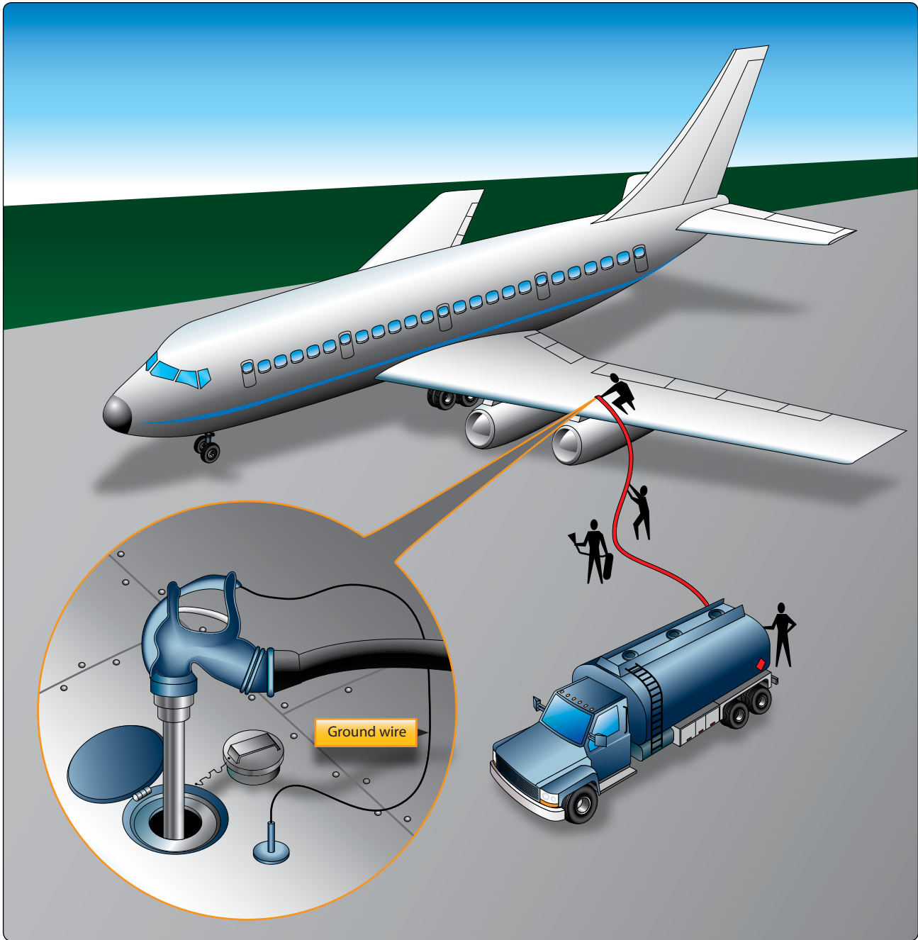
Figure 1-32. Refueling an aircraft by the over-the-wing method.
