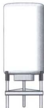
Chauffe-eau vertical (sur pied)
