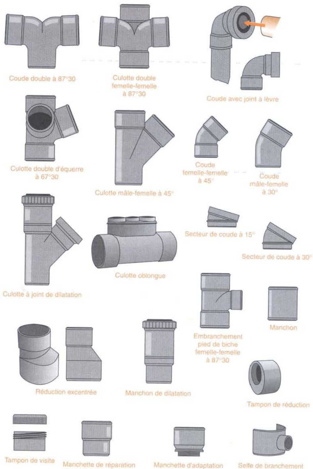
Figure 87 : Les raccords PVC
