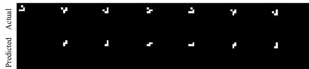
Figure 4: Predictions generated by a PredNet trained only on the exact sequence shown here. In this case, training data and test data are equal. Even for this simple task, PredNet seems to only be able to imperfectly predict the pattern, with a constant one-cell mistake. In reality, it seems that what was learned was a simple translation of elementary patterns of period 5.
