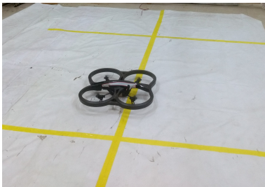
Fig. 14: Experimental setup for AR drone's PID tuning on grid lines using roll, pitch and yaw as control variables
