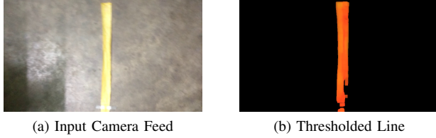
Fig. 5: Line Thresholding in HSV Space using SVM
