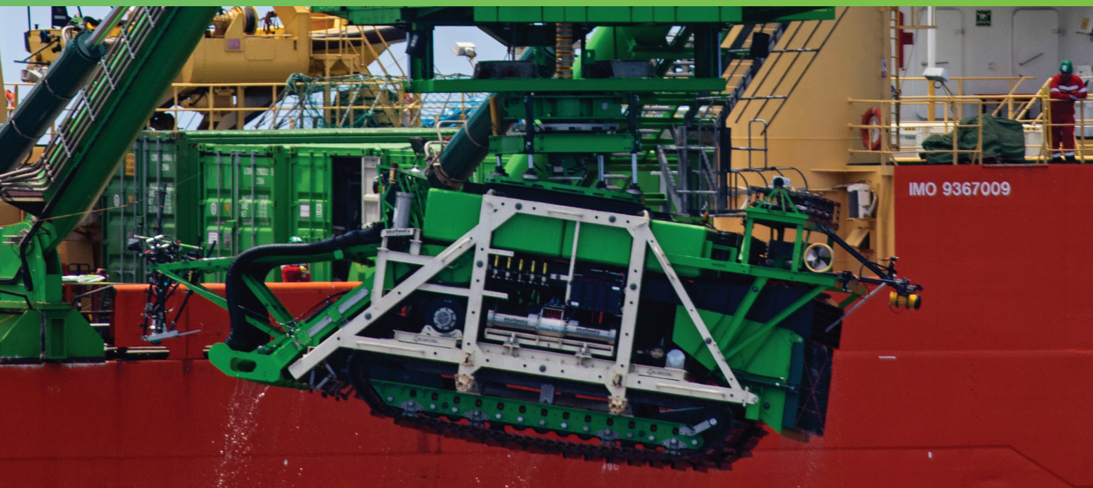
A nodule collector is launched during mining gear testing in the Pacific.
